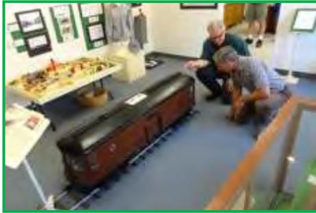
John Mercurio, pictured here). The model "interurban" car is fully functioning, and has 24 Volt, DC motors on each of the four wheels. Everything on this scale model is accurate, including the bell.
